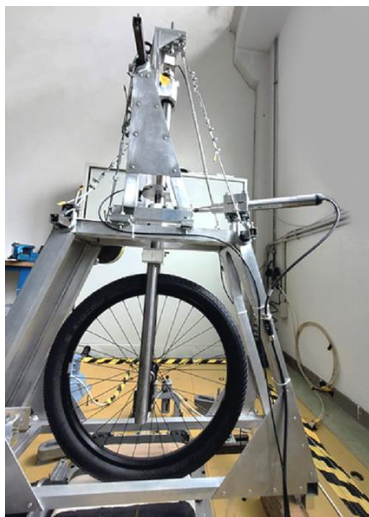
Figure 1. Test-rig VeTyT at Politecnico di Milano. It can be used to measure tyre lateral characteristics, as tyre parameters vary.
