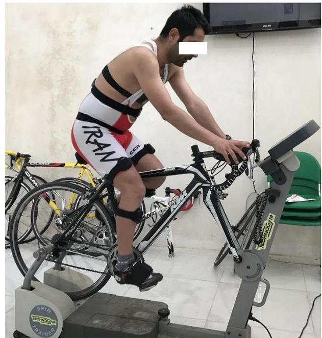
**Figure 1.** the depiction of a subject on the bicycle attached to Technogym ergometer and the location of myoMotion sensors on segments
