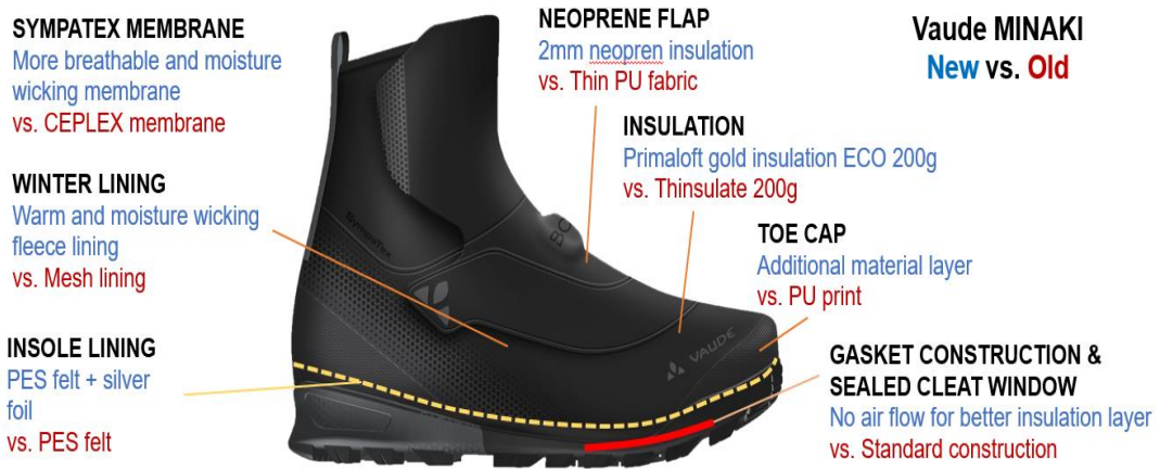
Figure 4. Differences in footwear between the new vs. old Vaude Minakt
