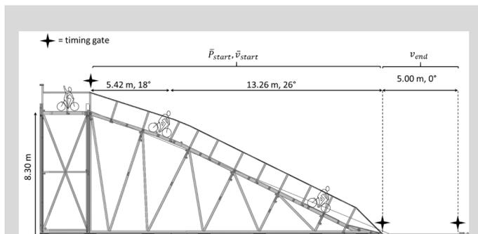
**Figure 2.** Diagram of the BMX 'supercross' starting ramp used during the study, showing the segments designated to determine mean starting velocity ( $\bar{v}_{start}$ ) and power ( $\bar{P}_{start}$ ) and for end velocity ( $v_{end}$ ).
