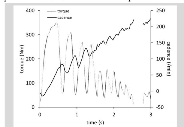
**Figure 4.** Example recording from a modified powermeter. Torque was measured with an SRM spider while pedaling cadence was measured with a gyroscope within an Axiamo data logger, which recorded both signals at 100 Hz.
