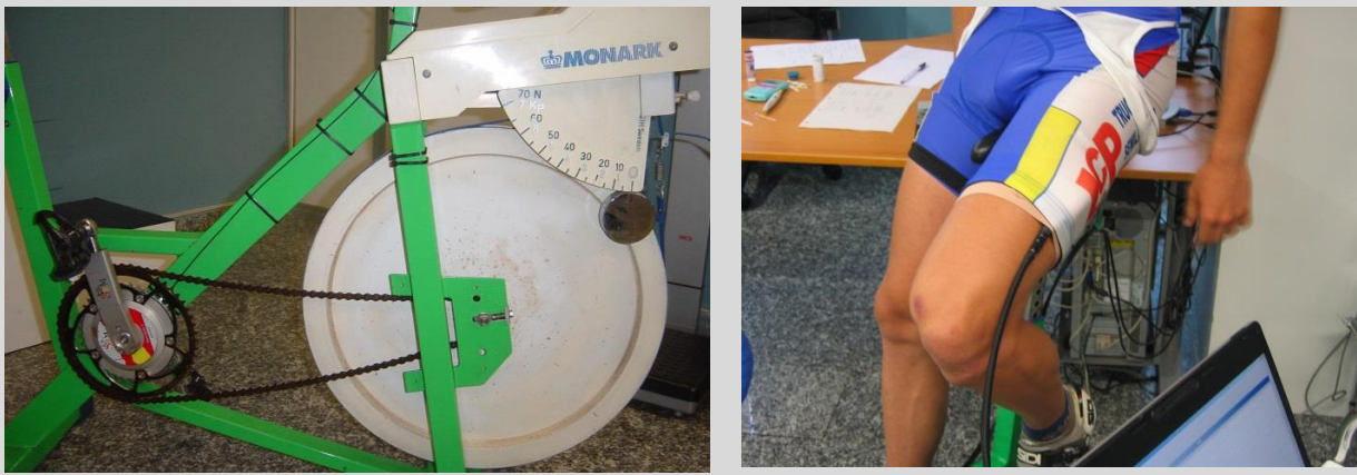
Figure 1 Experimental set-up. Left panel: modified Monark 818 modified. Handlebars, saddle and pedals are race bike type. The work load is settled by the mechanical brake and measured by the SRM system. Right panel. The NIRS probe is firmly attached to the shaved thigh by Tensoplast and covered by the race type short.
